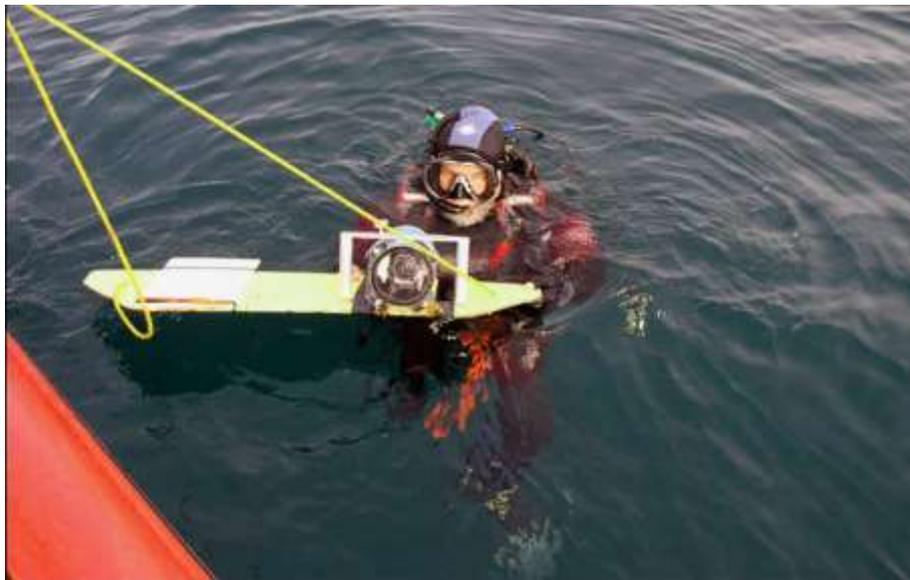
*Figure 5 Manta board fitted with video camera*
