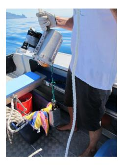
Figure 2 Drop video apparatus.
