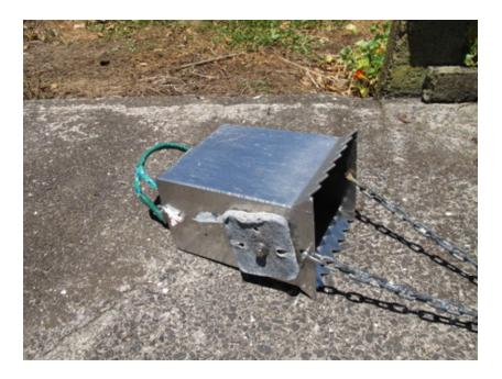
Figure 2. Box dredge used for this survey.
