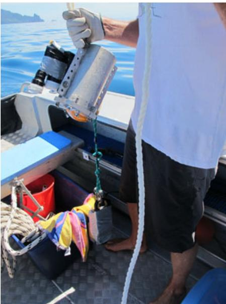
**Figure 2** Drop video apparatus.
