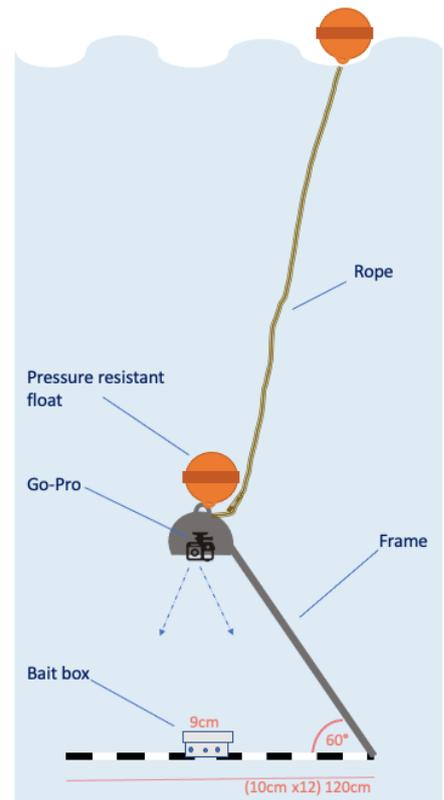
**Figure 4.** Diagram of a deployed BUV apparatus.
